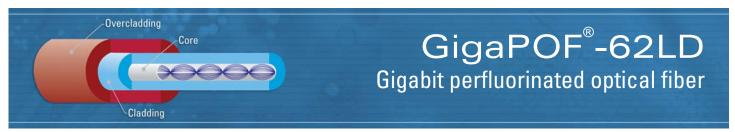
GigaPOF-62LD is a low attenuation, IR-transparent POF with higher bandwidth than any other type of plastic optical fiber. With a 62-micron core diameter, it easily couples to standard multi-gigabit transmitters and receivers, and the 750-micron outer diameter makes this fiber extremely robust and simple to handle. The combination of performance and simplicity makes this our most popular fiber for use in active cables and multi-gigabit data networking.
