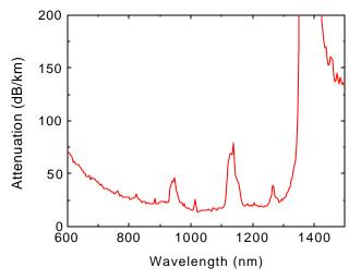
Attenuation typically 25-35 dB/km at 850 nm
