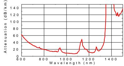
10-fold lower attenuation than PMMA-based POF IR transparency as well as visible transparency
