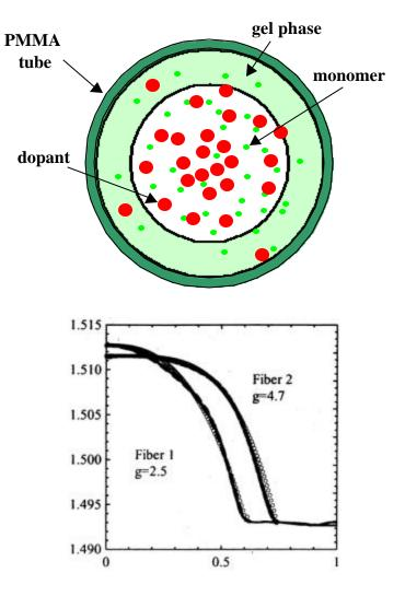
Interfacial gel was first effective graded-index POF technology Recently commercialized by Fuji Film Process has not been demonstrated with perfluorinated materials
